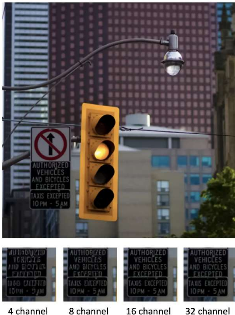
Figure 3. Autoencoder. The visual quality of the reconstructed images for autoencoders with different channel sizes. While keeping all other architecture layers the same, we only change the latent channel size. We show that the original 4-channel autoencoder design [27] is unable to reconstruct fine details. Increasing channel size leads to much better reconstructions. We choose to use a 16-channel autoencoder in our latent diffusion model.
